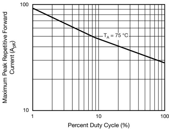
Fig. 3 - Maximum Peak Repetitive Forward Surge Current
